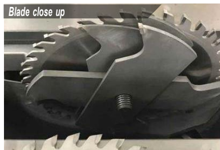
Install dado set as shown to prevent chipper jamming.
