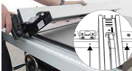
Position fence to access adj. screws
