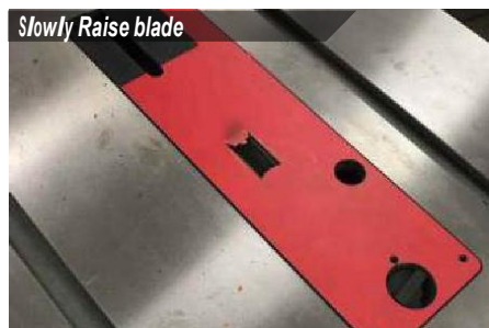
As the blade rises, the throatplate section will cut away. Stop the process at the desired blade height for application with the blade or dado set.
