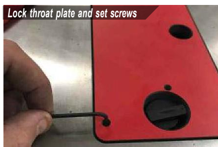
Lock the throat plate in position and screw in the Alan set screws so that the table tries to force away and comes in contact with the locking mechanism. This will ensure that the throat plate will not move and stays in the same location during the next steps.
